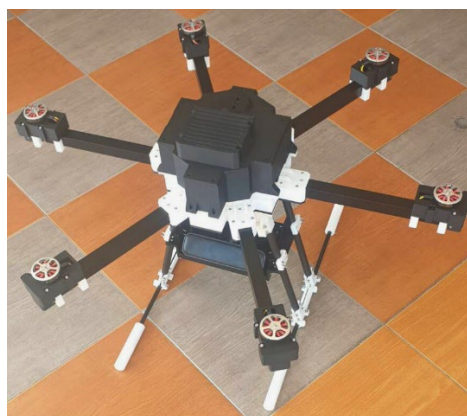
Figure 5 The completed prototype of the semi-autonomous hexacopter for real-time operation.
