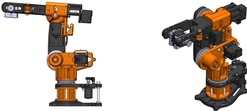
Figure 4 Side and Isometric Views of Robotic Arm.
