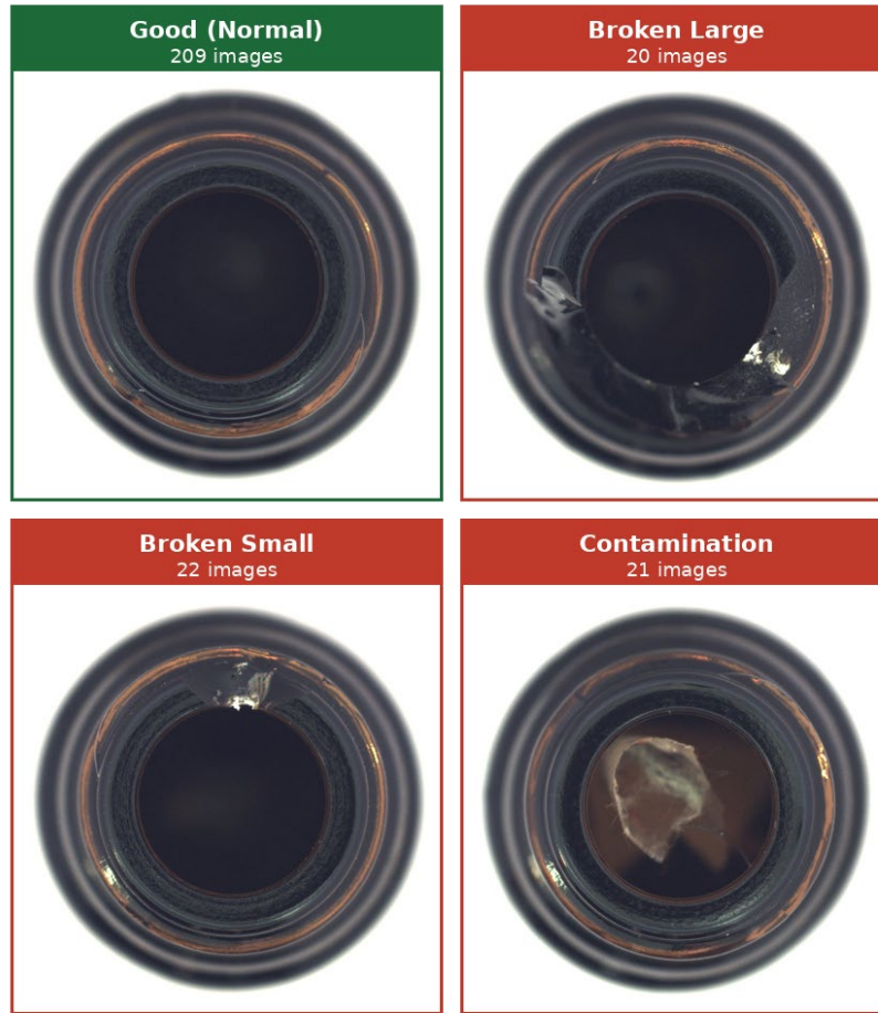
Figure 2 Defect Types in Glass Bottles (MVTec Dataset)
